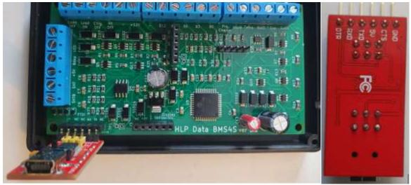
To the right you can see how the pins shall be located on a suitable FTDI-adapter
