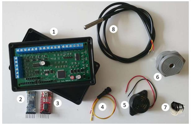
The basic package contains: 1: a BMS4S circuit board and a box to mount it in.
