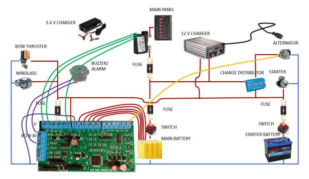
The simplest way is to just replace the main battery with LFP cells, and connect them to BMS4S. You also connect a buzzer/alarm to it. Then you move the voltage sense (often yellow) cable and connect it to BMS4S. You also have to connect a bi-stable relay between the new main-battery and to BMS4S. Then at last you connect the power to supply BMS4S from after the main switch (but before the relay) so it is switched off when all other electricity is switched off.
